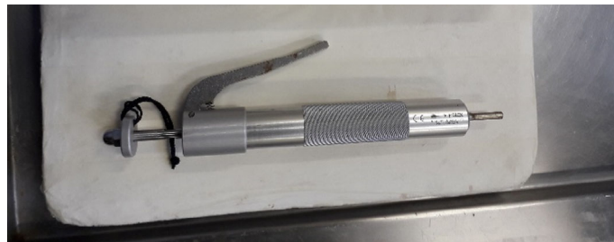
Figure 12: Example of a spring-loaded captive bolt. Source: kindly provided by Velarde A.
