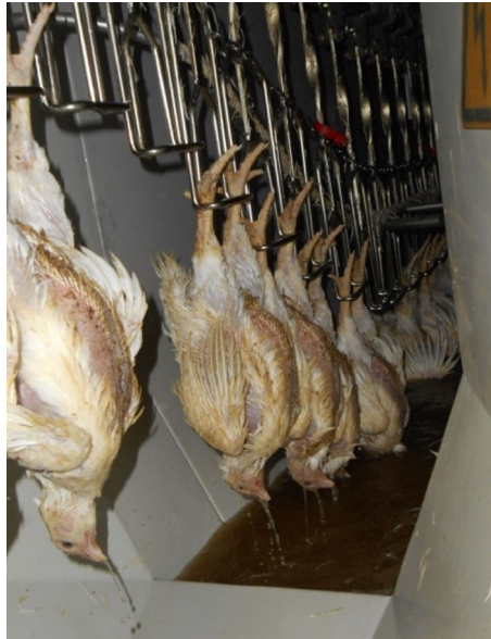
Figure 3: Illustration of waterbath stunner that can be used for on farm killing of poultry. Source: kindly provided by Berg C
