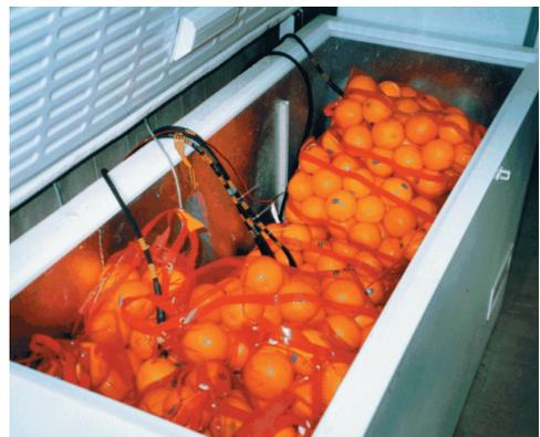
Figure 2. Refrigerator with fruits introduced into net bags.
