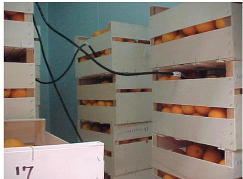
Figure 5. Storage of the fruits in the large-scale test and location of the temperature sensors at different plans.
