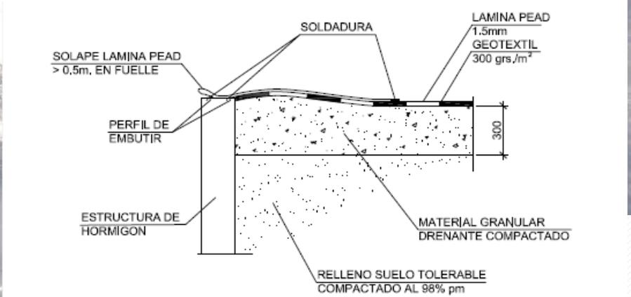
**DETALLE REMATE GEOMEMBRANA EN ESTRUCTURA DE HORMIGON**
