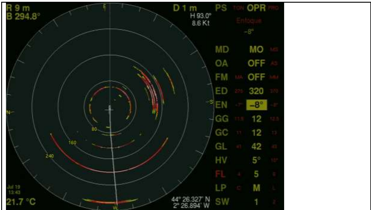
Figure 2: Example of detection of a bluefin tuna school by omnidirectional sonar (right part of the sonar screen).
