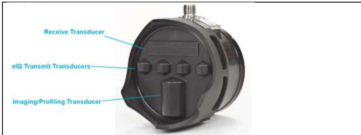
Figure 4: M3 mutibeam sonar used for complementary size measurements
