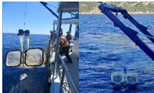
Figure 2. Bongo 90 and 20 samplers used in TUNIBAL cruises.
