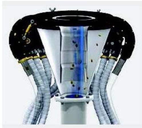
**• *IDS distributor system for Pöttinger Aerosem 1002 pneumatic seed drill.***
