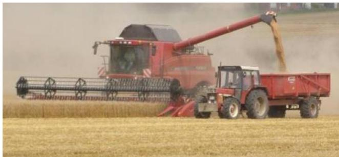
**• Pivoting unloading spout for Case-IH Axial Flow harvesters.**
