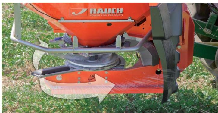
**• System to measure and adjust spreading in the Rauch AXMAT centrifugal fertilizer spreader.**
