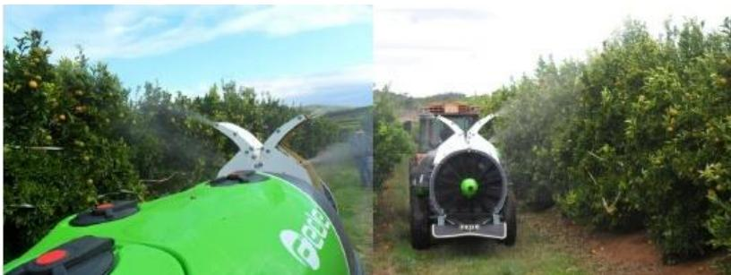
**• System for modifying the fan-driven air flow in Fede Futur Smart Air sprayers.**
