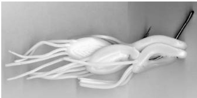
FIG. 2. FOUR LURES (ARTIFICIAL BAITS) JOINED TOGETHER, FOR TESTING ATTRACTIVENESS TO SEA TURTLES.
